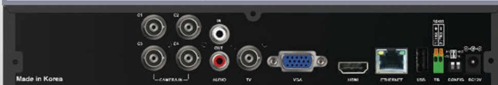
•HD-TVI Compact 4 channel DVR back of the DVR
